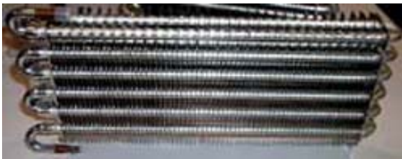
Figure 13 Air Cooling Condenser
